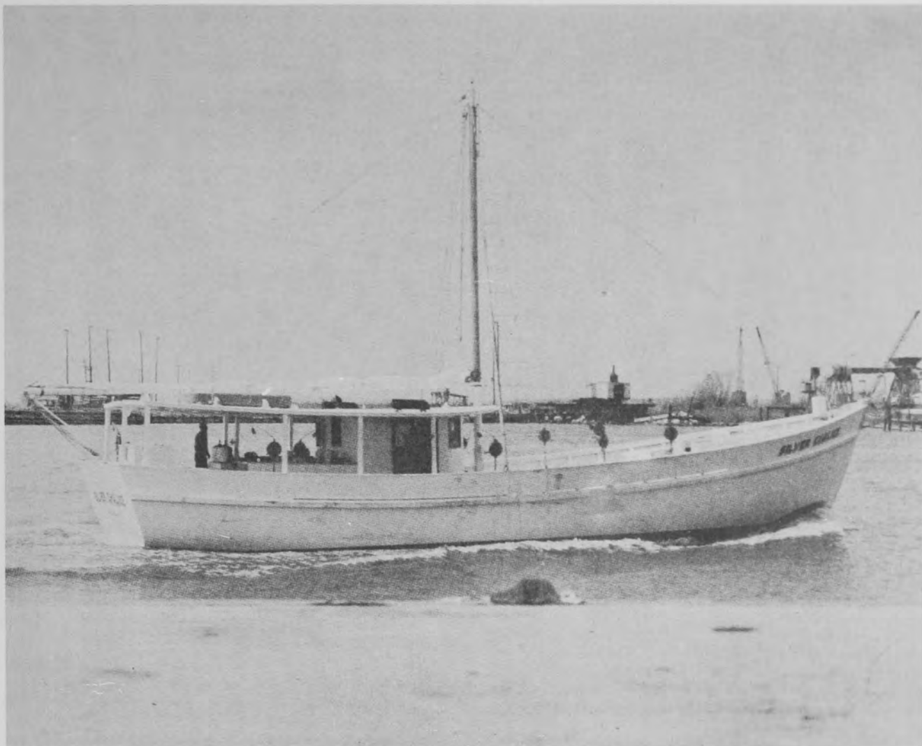
Figure 3.--The Silver Chalice , built in 1964, is a 63-gross ton, 72-foot snapper boat.
