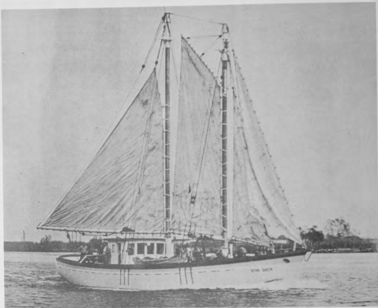
Figure 2.-- The Star Queen , built in 1953, is a 71-gross ton, 68-foot motor sailboat.
