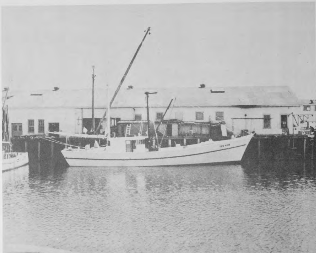
Figure 4.--The Ten Kids , built in 1964, is a 58-gross ton, 70-foot combination vessel that can be used to fish for snapper and trawl for shrimp.
