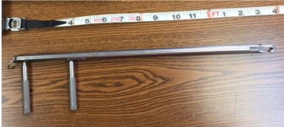
Figure 2.1.3. Example of new sea turtle release gear ‘hookout’ to release incidentally hooked sea turtles. Photo credit: NMFS-SEFSC.
