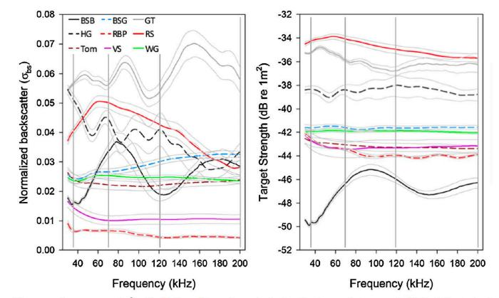
**Fig. 6.** Species specific averaged  $\sigma_{bs}$  response (m<sup>2</sup>) with 95 % confidence intervals (broken lines) around the mean (solid line). Vertical reference lines represent nominal operating frequencies in fisheries acoustics (38, 70, 120, and 200 kHz).
