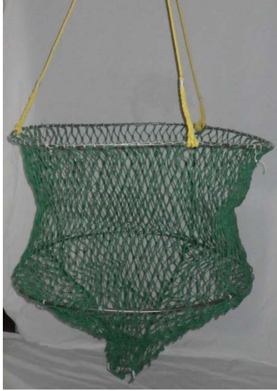
Figure 1.1.1. A collapsible net that can be used on-board and subsequently release incidentally hooked sea turtles.
