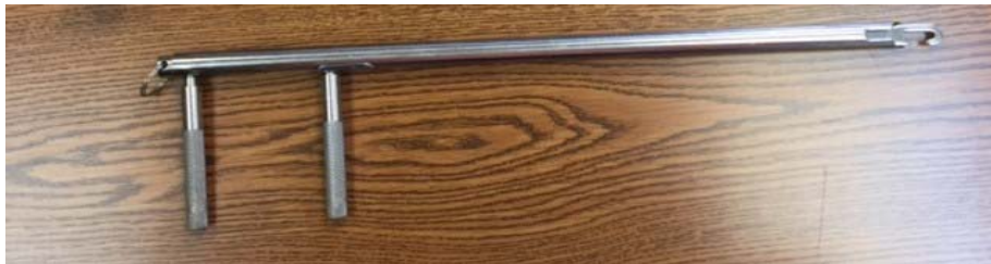
Figure 1.1.2. Example of new sea turtle release gear “Hookout” to release incidentally hooked sea turtles.
